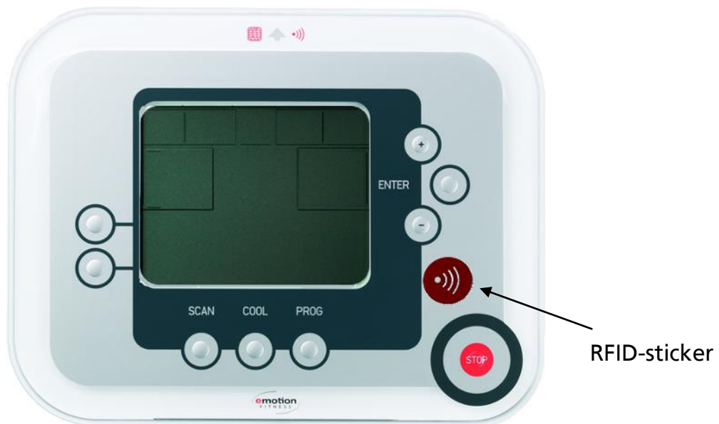
Fig. 5: RFID-button for RFID identification, in case the medium cannot be read via the slot
